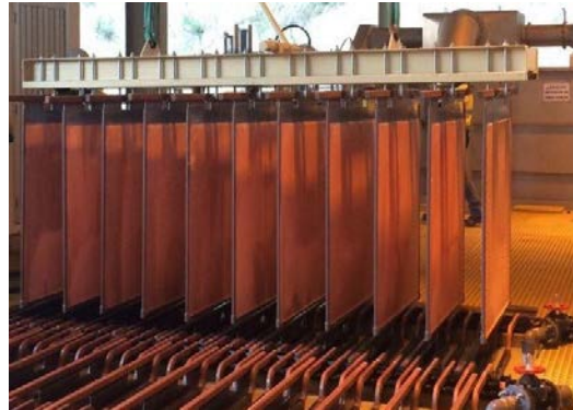
Copper Metal Plates on Cathodes
