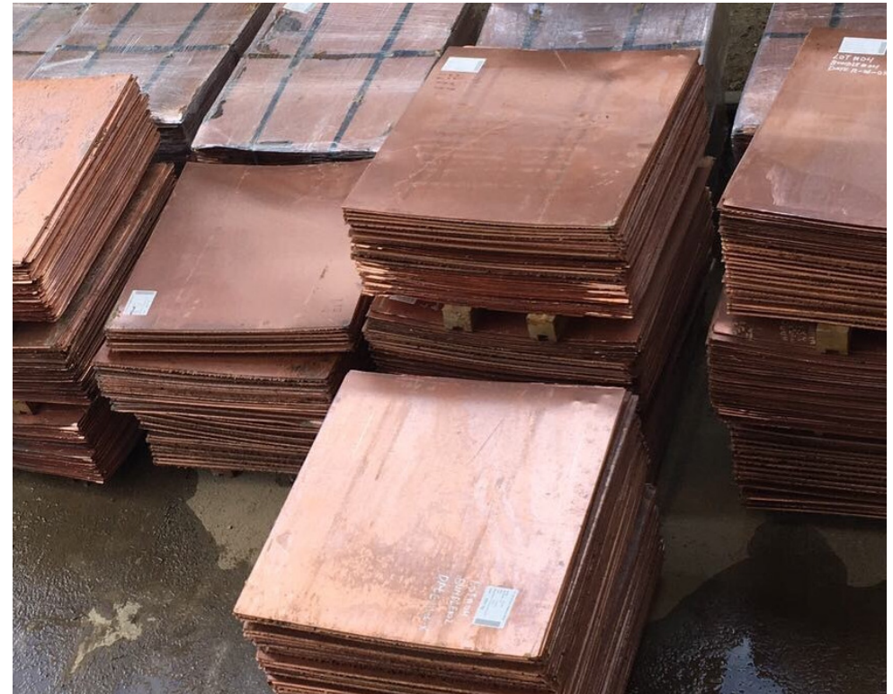
Wetar produced final LME Grade A copper metal (>99.99%) cathode onsite
